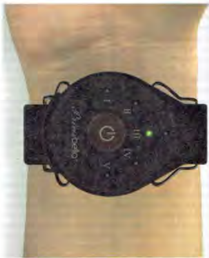
FIGURE 21-1 PrimaBella is a noninvasive transdermal device cleared by the FDA for the treatment of pregnancy-induced nausea and vomiting (morning sickness). The device is applied to the ventral side of the wrist, where the median nerve is closest to the surface of the skin. It emits a programmed pulse that stimulates the nerve to create electrical signals that travel to the central nervous system to restore normal gastric rhythm.
