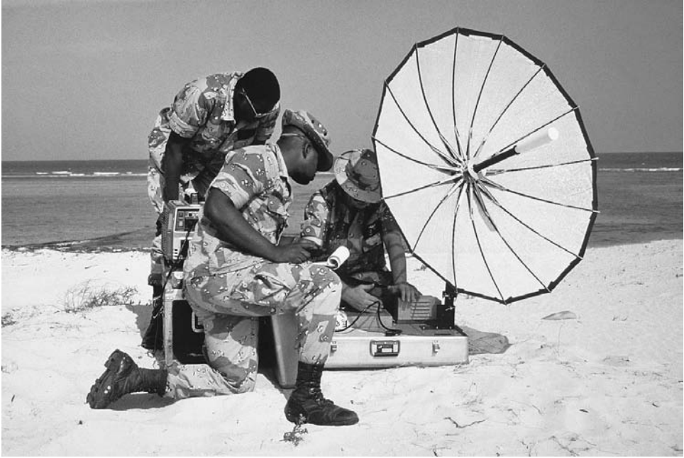
An Aerospace Audiovisual Service crew of videographers and photographers set up an Inmarsat satellite transmitter on the sand during Operation Desert Storm in Saudi Arabia. (Courtesy U.S. Department of Defense)
