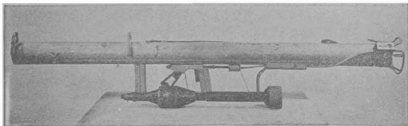
The Ofenrohr , with the projectile used in it and in the Püppchen .
