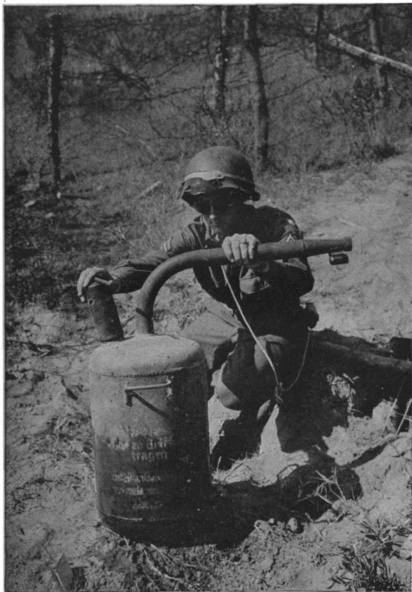
A fougasse flame thrower which has just been lifted from its emplacement.
